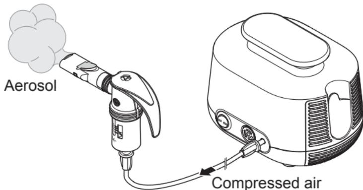
The compressor supplies the nebuliser with compressed air. When compressed air is supplied, the nebuliser generates an aerosol from the liquid, for example the medication with which it is filled. This aerosol is breathed into the lungs through the mouth-piece or optionally a mask.
